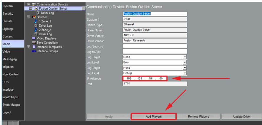
2. Check each Fusion Ovation Player driver in the Sources. Each one should have the server’s IP address as well as a unique Player MAC Address and Name. You can change the Name but should not change the MAC address as this is what determines which player the driver is controlling.
