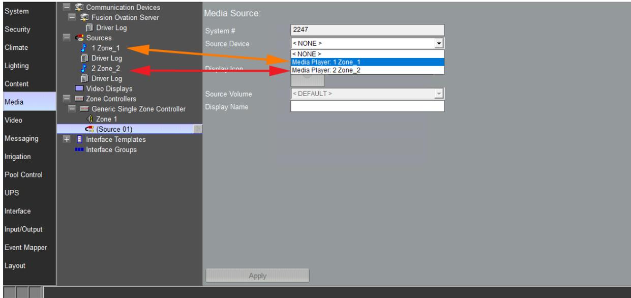
In this very simple example, you should have added one Server driver under the Communication Devices and one or more Player drivers under Sources. Each of the Player drivers should be connected to as a source inside your zone. Don't forget to hit Apply for these changes to take effect.
